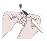
Place (test) indicator into a package that is similar to the typical packs used (e.g., in an autoclave bag) and in the area of the autoclave that is the most difficult to sterilize, i.e., over the drain or in the center of a full load. Run cycle.
