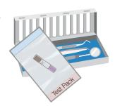
3 Caution: After sterilization, the contents of Attest biological indicators are hot and under pressure. Always allow to cool. Failure to cool for at least 10 minutes may cause the glass ampule to burst which may result in injury from flying debris.
